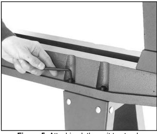
Figure 5. Attaching lathe unit to stand.
